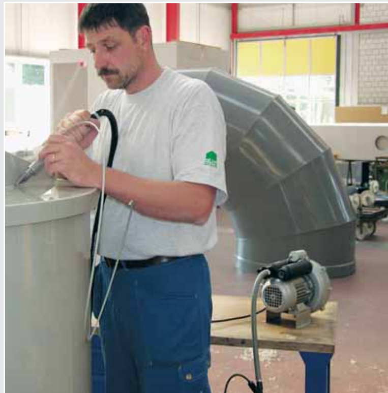
Blower ROBUST as air supply for the WELDING PEN.
