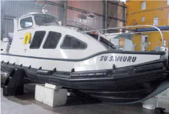
Ship constructed completely of HD-PE, Turkey
