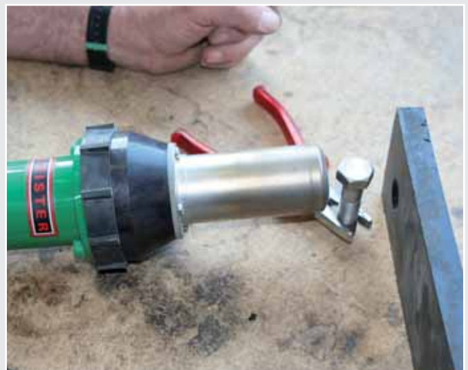
Heating a hex bolt before plunging.
