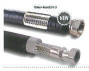
Hose Type Hose Material Braiding Material Fittings Materials Fittings Type Insulation Material Standard corrugated metal hose EN ISO 10380 Stainless Steel AISI 316L Stainless Steel AISI 304 (Braiding is optional) Carbon Steel St. 37.2/Stainless Steel Female-Male Rubber based special insulation (9-13 mm) Cryogel X201 (Aspen Aerogels) (5-10 mm)
