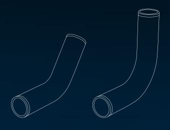
The LOKRING elbows are made from copper tube in accordance with EN 12735-1and suitable for an operating pressure up to 50 bar (725 psi).
