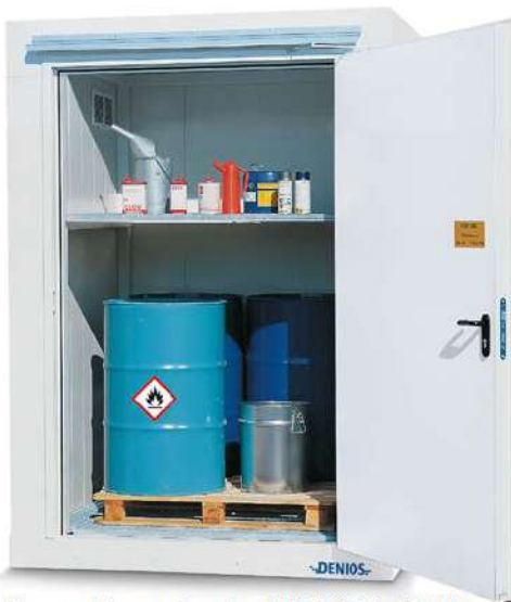
Fire-rated Storage Container BMC-S 180-2 with E190 door, for 2 x 205 litre drums and shelving for small containers (optional)
