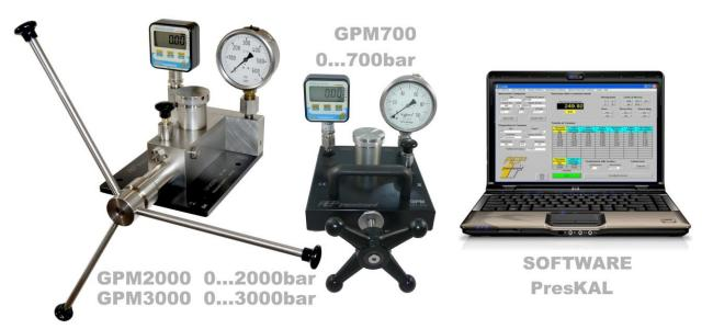
Manual pressure generators used to compare the measurements between the sample pressure gauge and the instrument calibration.
