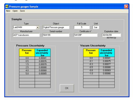
On this page are stored all data on standard instruments that can be used during the calibration.
