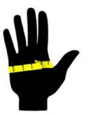
In order to determine the proper size for Class 0 and 00 insulating gloves, use a tape measure to find the circumference of your hand around the palm.
