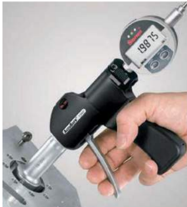
Output jack enables collection of measurement data for SPC analysis
