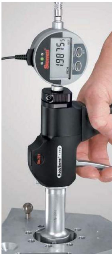
Output jack enables collection of measurement data for SPC analysis
