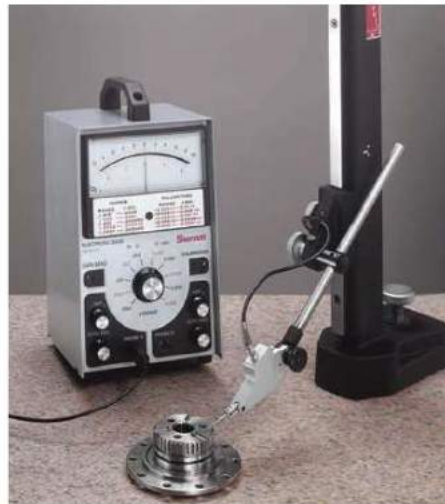
717 Electronic Gage Amplifier with 252 Transfer Gage and 715-1Z Gaging Head
