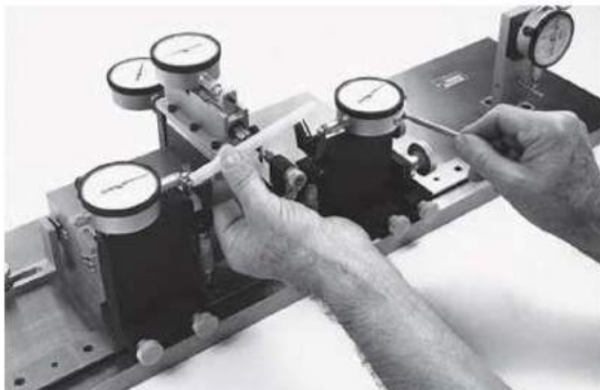
Inserting ceramic cylinder in gage to check squareness and parallelism of ends, longitudinal bow and out-of-roundness
