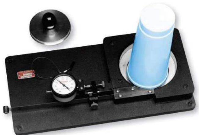
Top of 1/2-gallon container in measuring position
