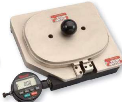
Master in position to set indicator to zero
