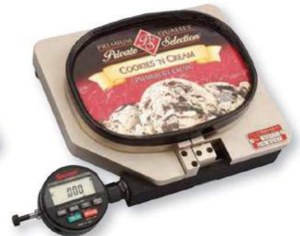
Top of 1/2-gallon container in measuring position
