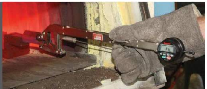
Variation on a theme: A large caliper with long reach for web thickness of train tracks hot or cold.
