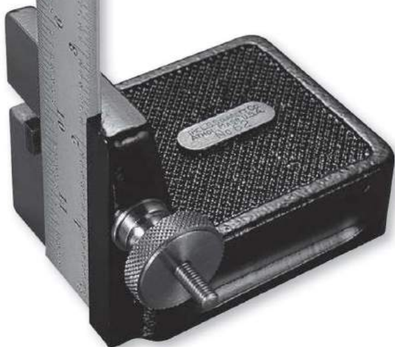
Transferring measurements with a Starrett Surface Gage used in conjunction with rule and rule holder
