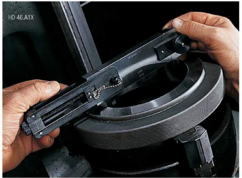
Snap gage is used to check inside dimensions of ring gage still mounted in internal grinder
