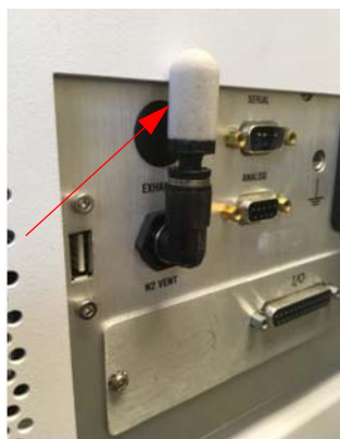
Figure 8-1 Dry Nitrogen Vent
