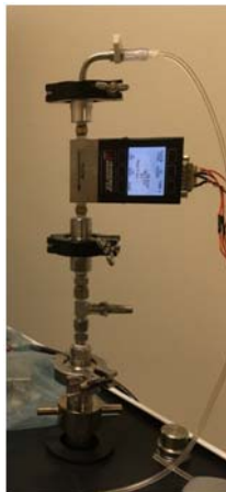
Figure 5-19 Alicat Scientific Mass Flow Meter Supported Method of PPM Testing
