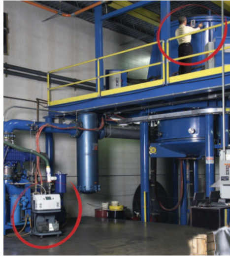
Figure 1. Leak detection of large volume vacuum chambers.
