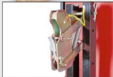
Gripper head with integral equipotential bonding - EX proof even in the smallest details
