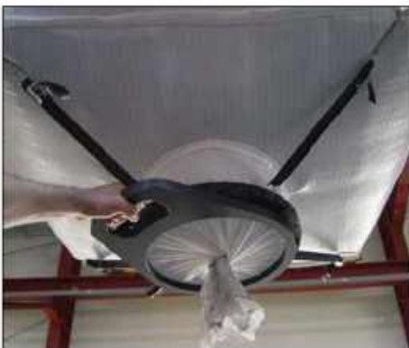
Big Bag outlet frame for manual operation, with 4 hanger straps and hooks
