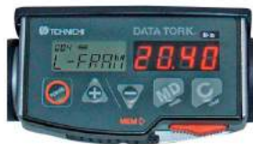
Display part Left: Part name, Right: Torque value
