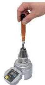
BMRD torque checking with BTGE-G.
