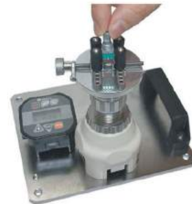
ATGE-G with table attachment and measurement stand
