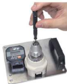
AMRD torque checking with ATGE-G and measurement stand, #808.
