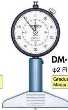
DM-220 / 230 Needle Contact point Graduation 0.01mm Measuring Range 20mm/30mm
