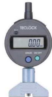
DMD-252S 2 φ3.2 Steel Ball Contact Resolution 0.01mm Measuring Range Concave 5mm Convex 4mm
