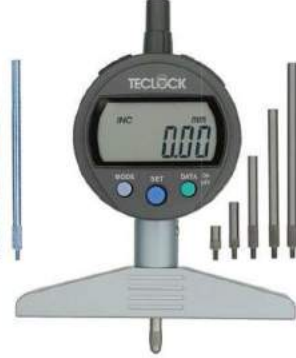
DMD-215J φ3.2 Steel Ball Contact Point Resolution 0.01mm Measuring Range 220mm Indication Range 12mm With 5-Extension rods
