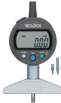
DMD-214J φ3.2 Steel Ball Contact Point Resolution 0.01mm Measuring Range 220mm Indication Range 12mm With 5-Extension rods
