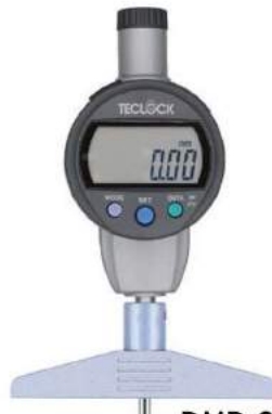
DMD-241J φ3.2 Steel Ball Contact Point Resolution 0.01mm Measuring Range 25.4mm
