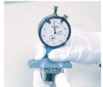
Measuring depth of concavity of work of which center is bored. The photo shows 2.03mm.
