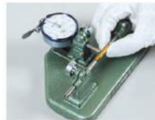
Measurement example for swing of round bar.
