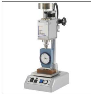
In order to solve individual difference of measured value, it is clearly mentioned in the standard to measure hardness by mounting durometer to stand.
