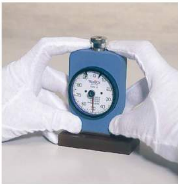
As to measuring hardness by pushing by hand, durometer to work piece form the top and read value by making pressed surface adhere to durometer.
