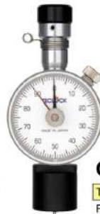
GS-709N Type A Durometer General rubber Soft plastic
