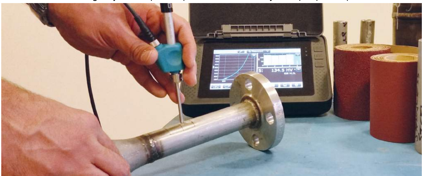
Figure 26: Performing Leeb measurements on test sample
