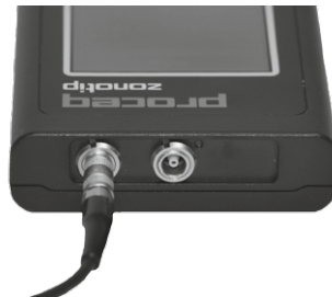
Figure 4: Connection of the 2.5 MHz transducer
