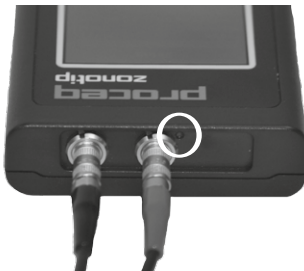
Figure 3: Connection of the 4.0 MHz transducer. Make sure the red cable is connected to the port with the red dot.
