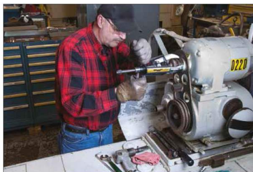
◀ Positioning an EP-104, 3-jaw puller on the drive pulley of an electric motor.
