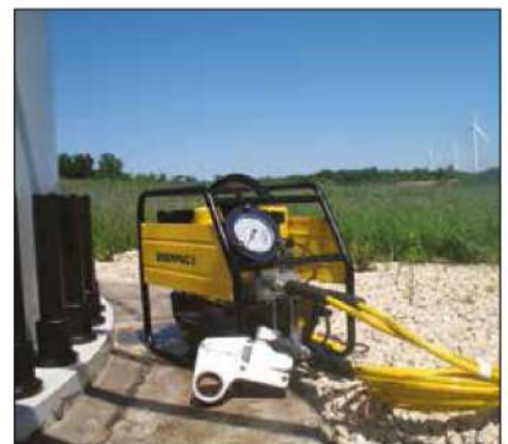
The TQ-700E and the W-Series wrenches are a productive combination in wind applications. ▶
