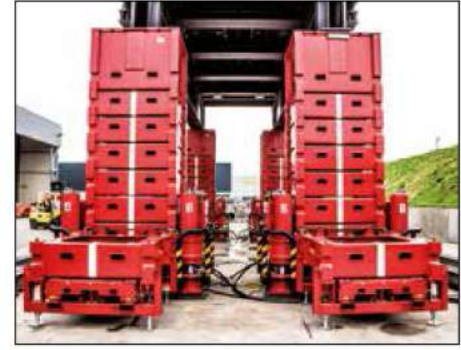
▼ Lifting barrels are stacked together to mechanically hold the load
