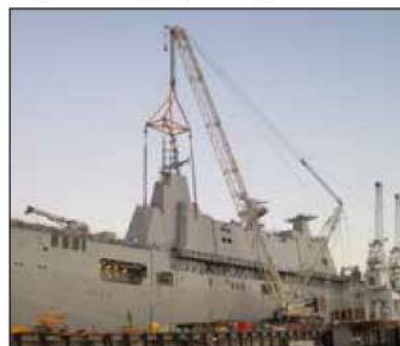
▼ An SyncHoist system used to align steel blocks of the ship's control tower sections allowing gradual lift and positioning of the load.
