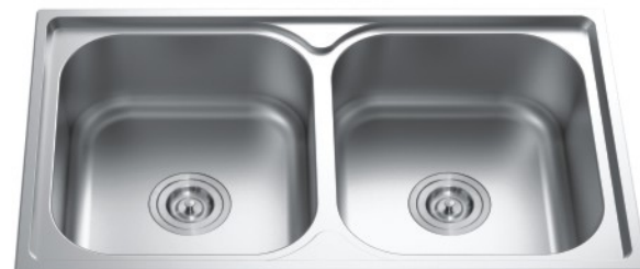
ERN 43020 Double Bowl (c/w Waste, Bottle Trap & Overflow) D: 820x485x230mm Material: 304 Stainless Steel Furnishing: Pearl Surface Thickness: 1.2mm Optional: ERN-OT-D25 (Basket)
