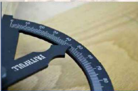
Laser etched graduations from 0 – 180° degrees.
