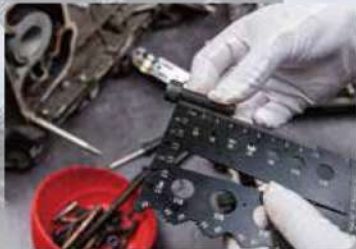
Gage Leg Quick-Check Perpendicularity
