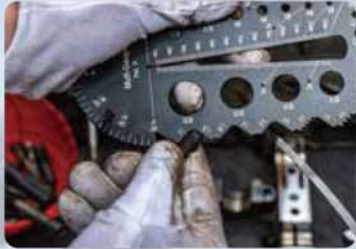
Pitch Size Measure the Thread
