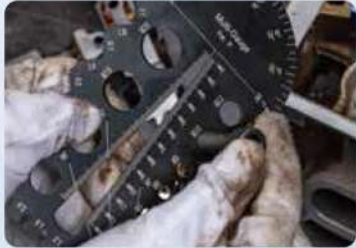
Gage Holes Measure the Major Diameter of Bolt
