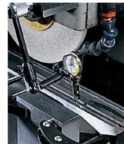
657A with 711LS Last Word Dial Test Indicator setting up workpiece on surface grinder.
