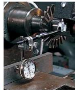
657A with 196B1 Universal Dial Indicator setting up workpiece on milling machine.
