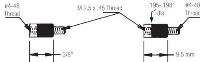
From Metric Racks to Inch Contacts PT24728
