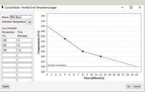
**Reference Batch**—store optimal cure reference profiles to compare measurement results
