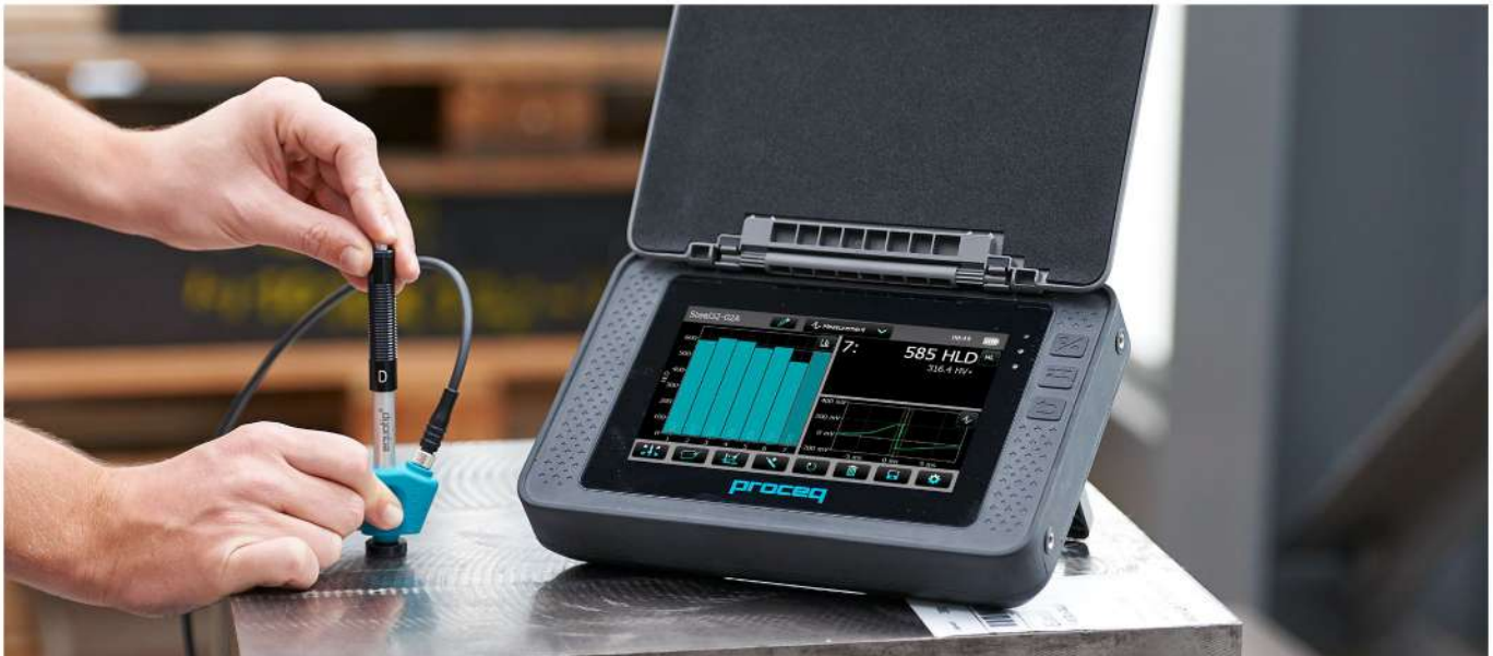
Figure 5: Equotip 550 Leeb hardness testing instrument
