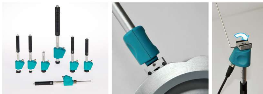
Figure 12: Overview of Equotip 550 Leeb Impact Devices and usage of support rings
