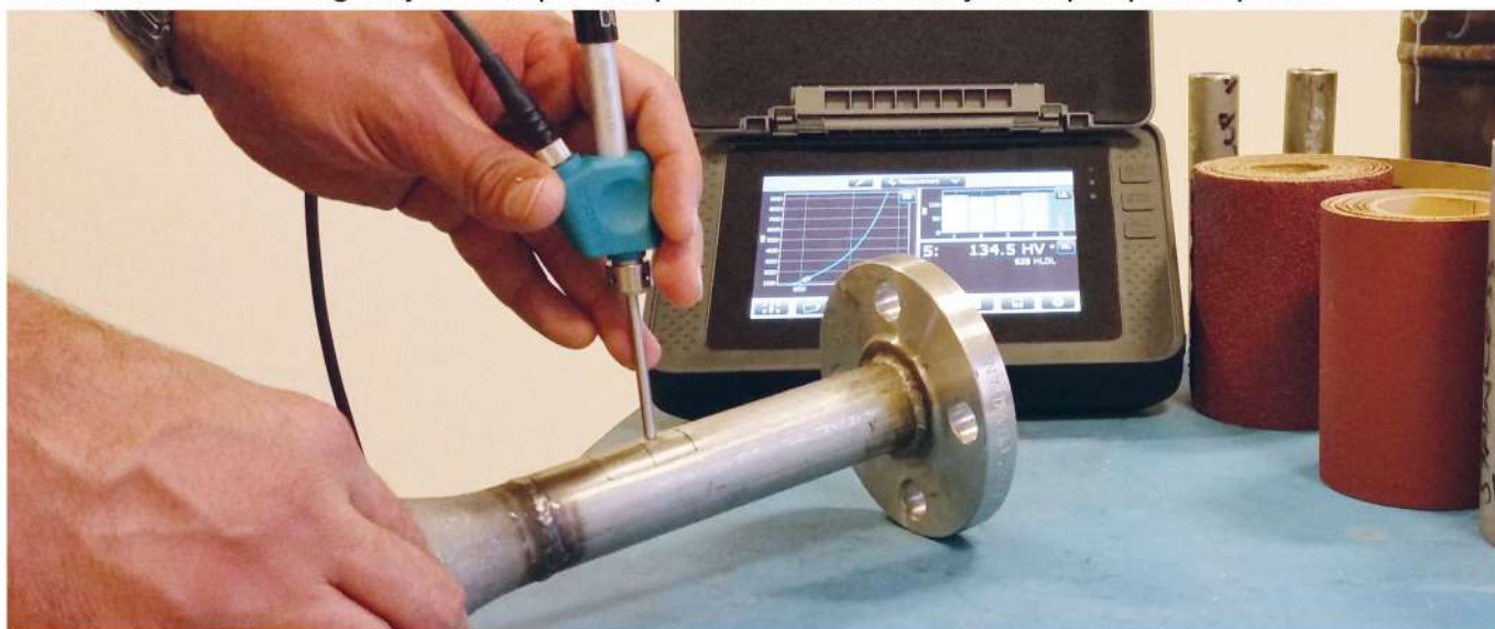
Figure 26: Performing Leeb measurements on test sample
