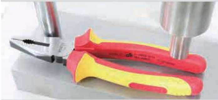
Handle passed impact resistance test
