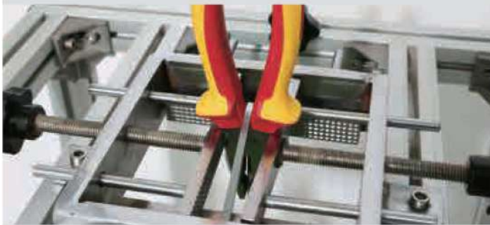
Handle passed 500N drawing force test
