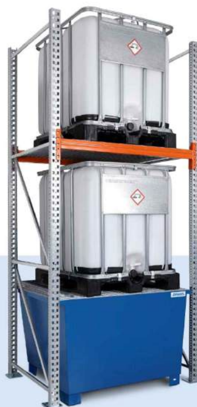
Hazardous materials pallet rack with 2 storage levels and painted spill pallet, basic shelf unit, compartment dimensions (WxD) 1400 x 1300 mm
