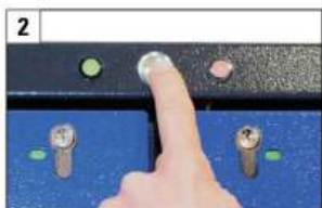
2 Operation indicator (green LED) and warning light (red LED)
