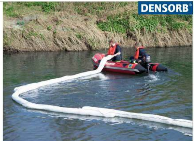
DENSORB oil barriers (here: 6 M sections) for containing and absorbing oil spills on water
