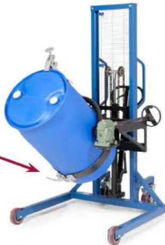
Safety clamp for plastic drums, with adjustable lever operated locking clamp
