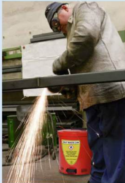
The self-closing lid prevents the content from igniting, e.g. by flying sparks
