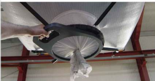
Big Bag outlet frame for manual operation, with 4 hanger straps and hooks
