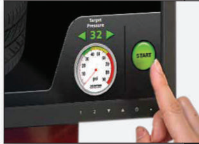
Blast inflation directs large blast of air for tough bead seating.
