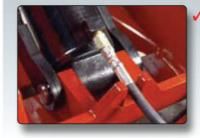
Instantaneous shutdown in event of hydraulic failure
