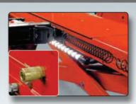
✓ Convenient air source for tools at front and rear
